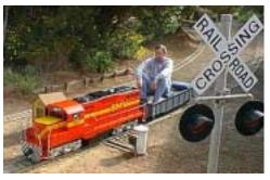
saying is, "This is pretty cool!" This No. 1801 is 1.6" to the foot and is powered by a V-twin, 16-horsepower gasoline engine that runs on regular gas. The engine runs a hydraulic pump which in turn runs hydraulic motors on each truck that drive each axle by chain and sprocket. This No. 1801 will be at SMVRHM's Choo Chew Saturday on May 17 (see page 1 article). Hop on board!
